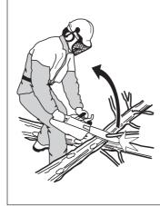
4 Never use the saw above shoulder height and try not to cut with the tip of the bar.
